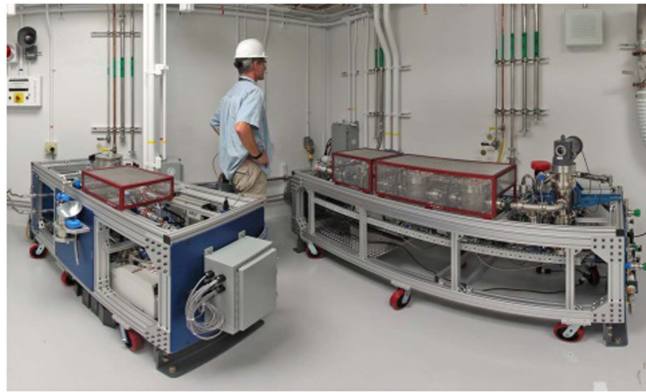
Figure 20. The ‘Radiochemical Analysis of Gaseous Species’ (RAGS) apparatus. The gas-load from the NIF chamber is pumped to RAGS following a shot where it is filtered to remove unwanted species (right cart) before the noble gases are cryogenically frozen and analyzed (left cart) to quantify the number of nuclear reactions that occurred during a shot. Reprinted with permission from [6]. Copyright (2012), AIP Publishing LLC.
