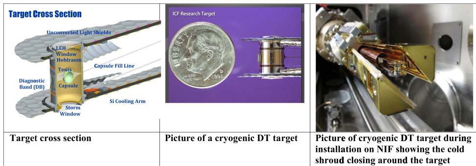
Figure 3. ICF target configuration at the NIF.
