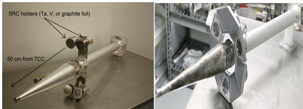
Figure 21. Solid radiochemistry (SRC) diagnostic. The standard SRC configuration (left) consists of four, 2 inch diameter collectors mounted on the end of a boom at a distance of 50 cm from the Target Chamber Center (TCC). The larger area vast area detector for experimental radiochemistry (VADER) (right) has a total surface area roughly six times larger than the four standard SRC foils combined. Left figure reprinted with permission from [113]. Copyright (2014), AIP Publishing LLC. Right figure reproduced with permission from [111]. Copyright 2015 Society of Photo Optical Instrumentation Engineers.
